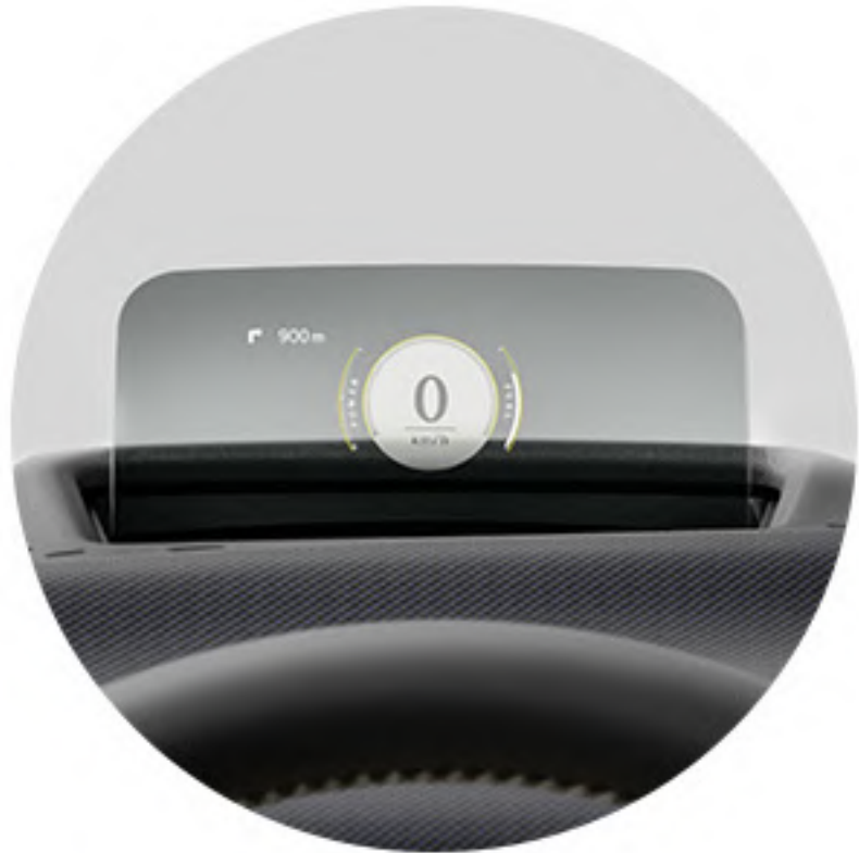
MINI Head-up Display: Display of Entertainment information, warning information & Driving speed.
